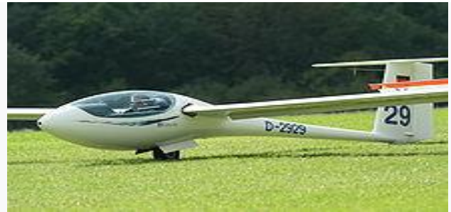
A Schleicher ASG 29 glider shows its monowheel landing gear
