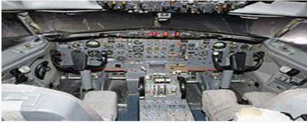
The nose gear steering-wheel (tiller) is visible as a semi-circular wheel to the left of the yoke in this photo of a Boeing 727 cockpit
