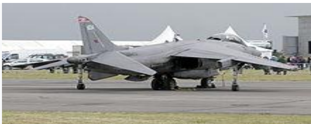
Hawker Siddeley Harrier GR7 (ZG472). The two main wheels are in line astern under the fuselage, with a smaller wheel on each wing
