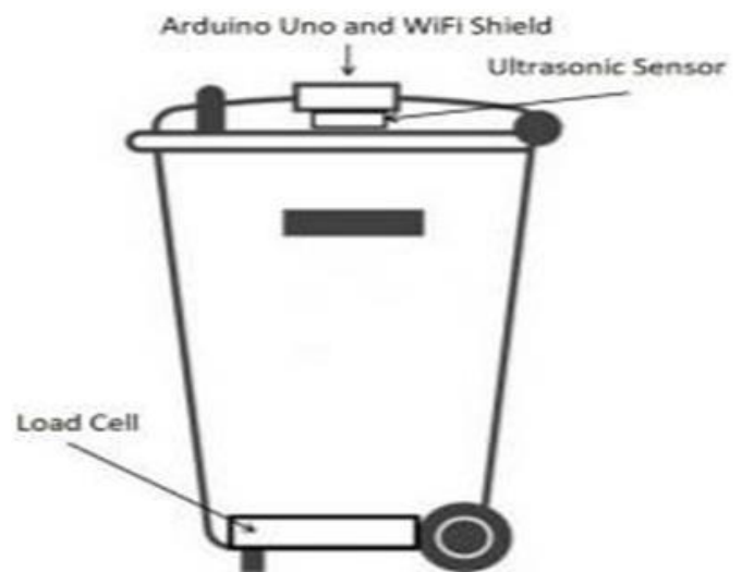
Figure 3.2: Sensor placement in the bin
