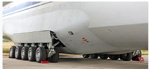
Oleo strut rear landing gear of an Antonov An-124 (24 wheel landing gear)
