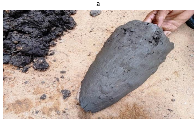
Fig 5 A : Roofing Tiles (Khapra) preparation
