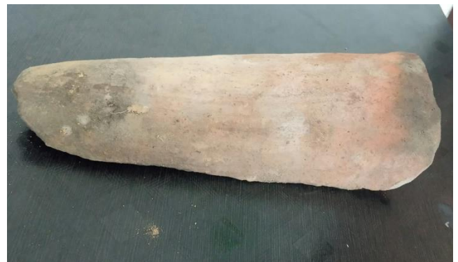
Fig 5 B : Prepared roofing Tiles (Khapra)
