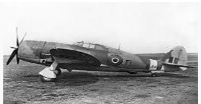
A Royal Air Force P-47 with its raked-forward main gear, and rearward-angled main wheel position (when retracted) indicated by the just-visible open wheel door.
