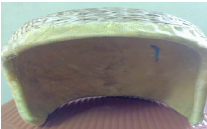
Figure 4: Bamboo Substrate Composite Helmet
