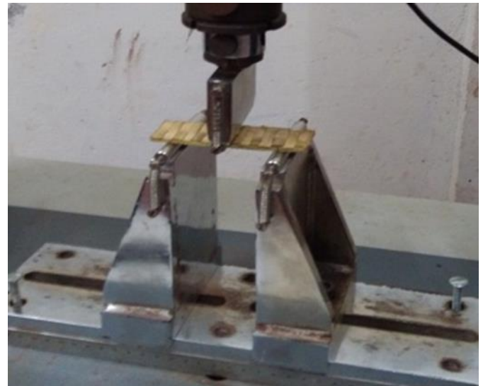
Figure 11: Bending Test on Helmet Specimen
