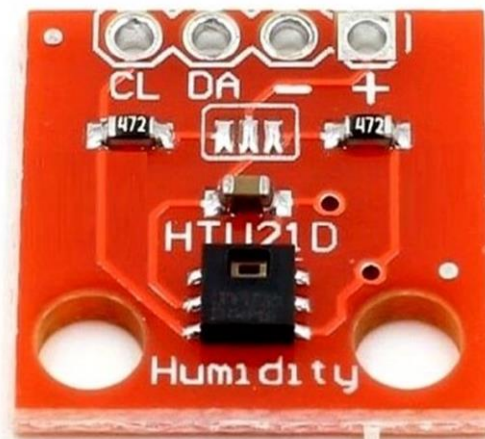
Fig 3: Temperature and Humidity Sensor (HTU21D)
