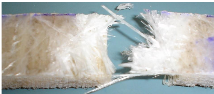
Fig.8. Fractured Impact Test sample
