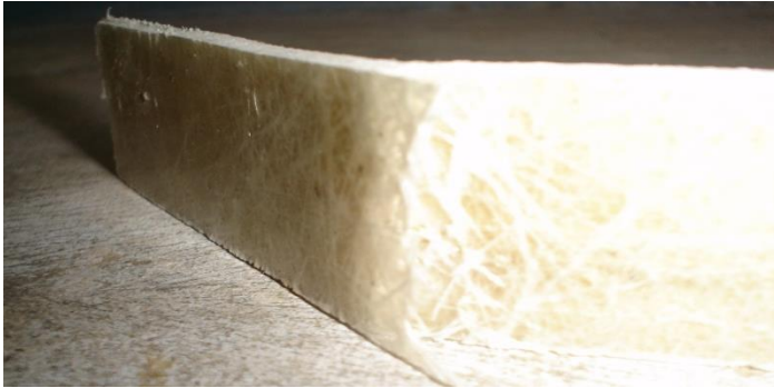
Figure 9 Impact Failure of the Specimen
