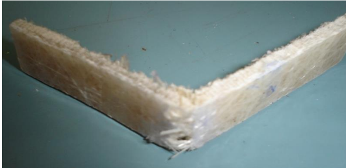
Figure 6 Flexure Failure of the Specimen
