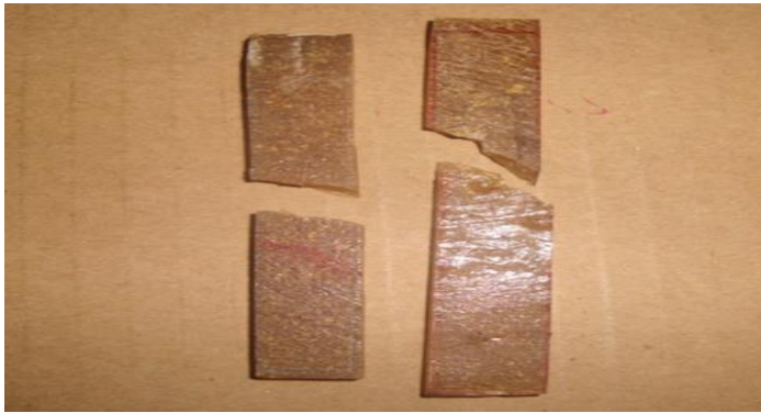
Figure 3 Specimen for impact test
